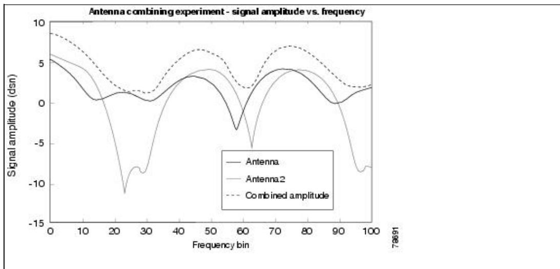
The actual received signal is a combination of a primary signal and several echoed signals. Because the distance traveled by the original signal is shorter than the bounced signal, the time differential causes two signals to be received. These signals are overlapped and combined into a single one. In real life, the time between the first received signal and the last echoed signal is called the delay spread, which can be as high as 4  $\mu$ sec.
