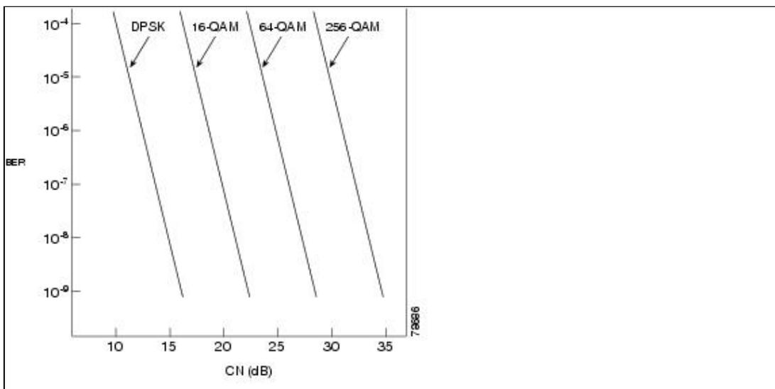
How the data is encoded also plays an important part in the equation. The data is usually scrambled, and a significant amount of forward error correction (FEC) data is also transmitted. Therefore, the system can recover those bits that are lost because of noise, multipath, and interference. A significant improvement in BER is achieved using FEC for a given SNR at the receiver. (See the [Figure: BER Against Signal-to-Noise for Coded and Uncoded Data Streams](#).)
