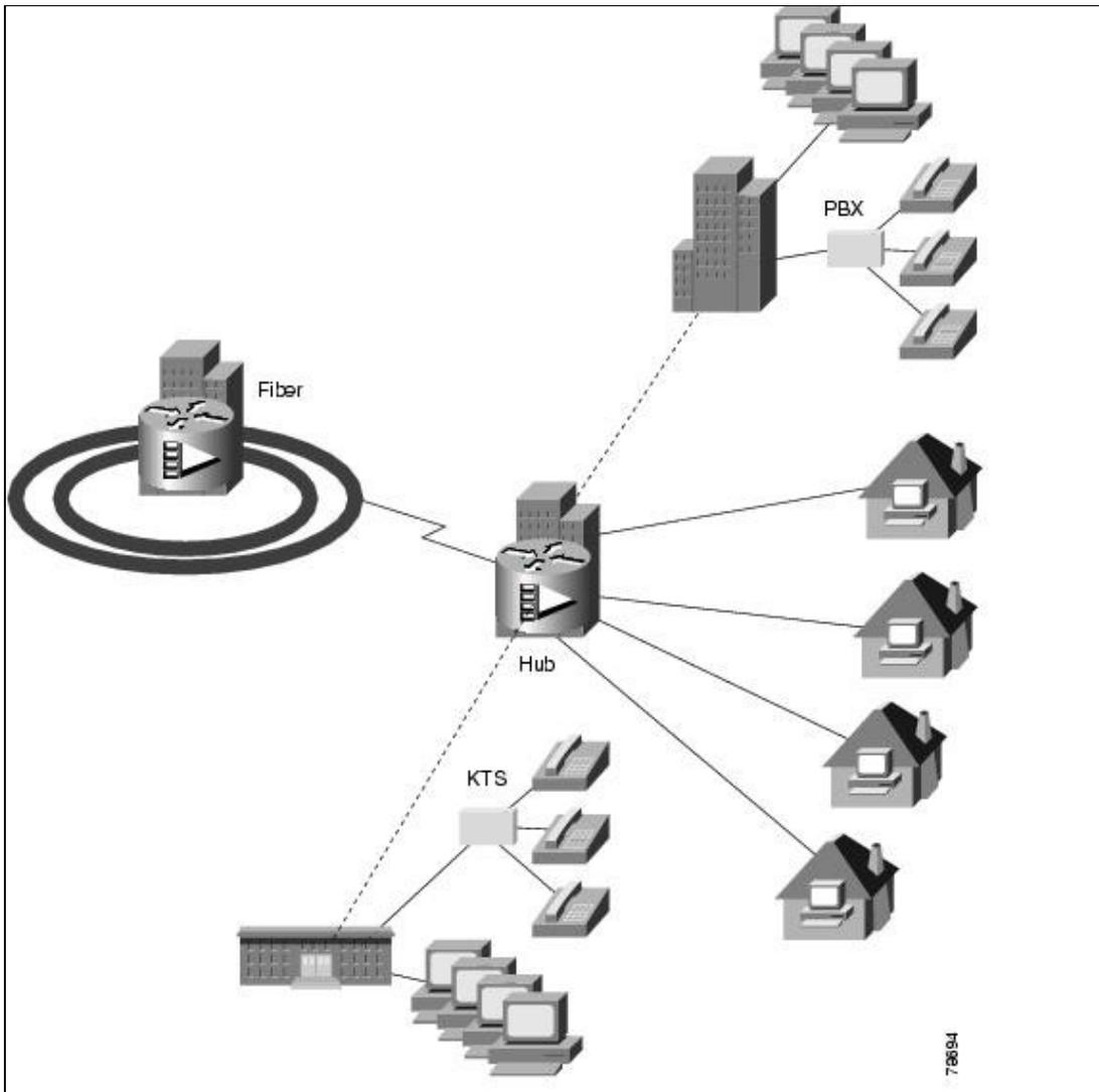
The P2MP wireless router will be an integrated solution. At the base station (or head end, or hub), it will consist of a base universal router (UBR 7246 or UBR7223), a wireless modem card, an outdoor unit (ODU) for the appropriate frequency band, cables, and antenna subsystems, as shown in [Figure: The Cisco MMDS Broadband Wireless Access System](#).
