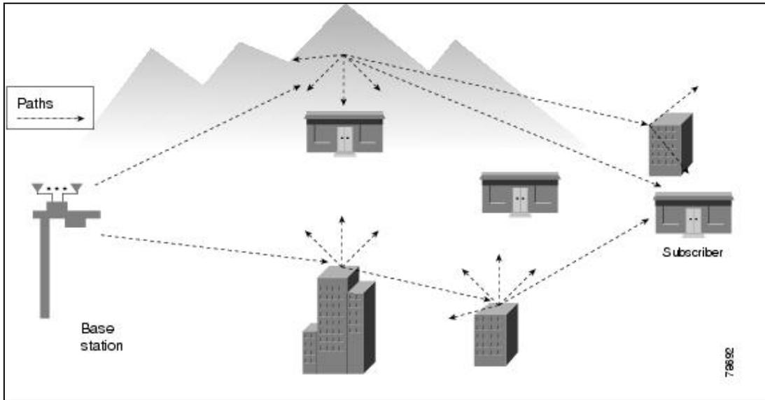
In analog systems such as television, this multipath situation can actually be seen by the human eye. Sometimes there is a ghost image on your television, and no matter how much you adjust the set, the image does not go away. In these analog systems, this is an annoyance. In digital systems, it usually corrupts the data stream and causes loss of data or lower performance. Correction algorithms must be put in place to compensate for the multipath, resulting in a lower available data rate.
