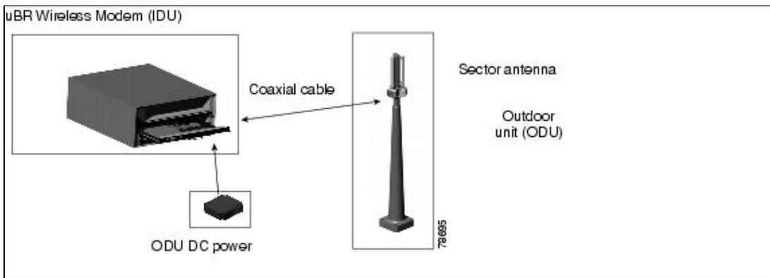
At the small business customer premises, the system consists of a network module in a 3600-family router, with an outdoor unit (ODU) and antenna. This CPE equipment is simpler and, therefore, less expensive than the head end (HE) equipment. The 3600 family has a wide variety of interfaces to match all types of customer equipment.
