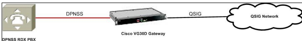
Figure 1: Cisco VG30D Voice Gateway.
