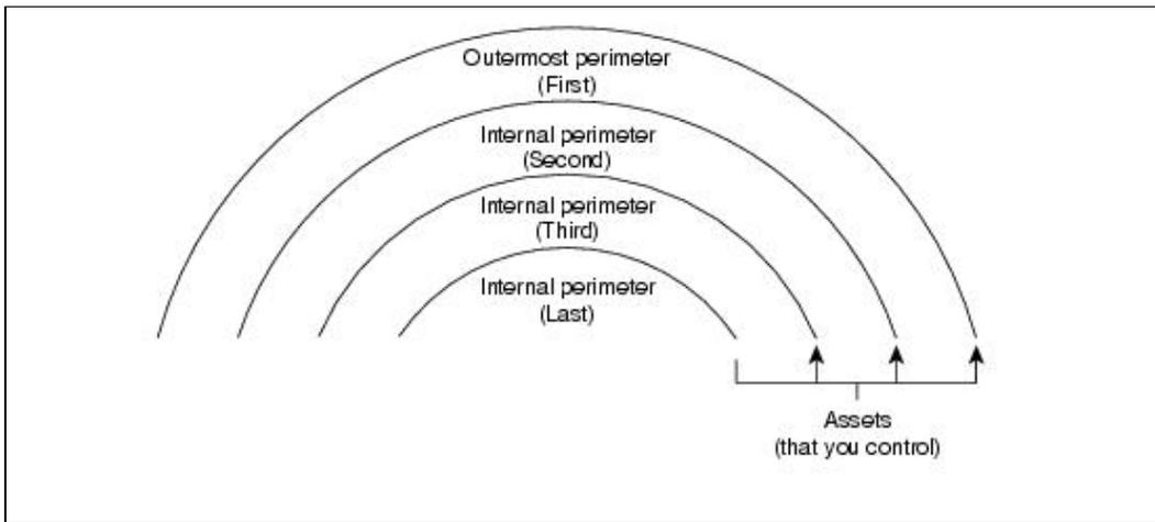
The outermost perimeter network identifies the separation point between the assets that you control and the assets that you do not control—usually, this point is the router that you use to separate your network from your ISP's network. Internal perimeter networks represent additional boundaries where you have other security mechanisms in place, such as intranet firewalls and filtering routers.
