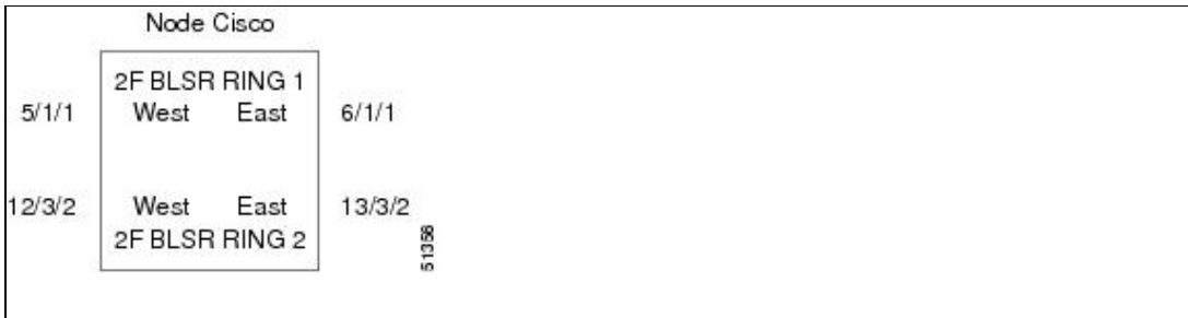
Figure 2-28: Two-Fiber BLSR to Two-Fiber BLSR
