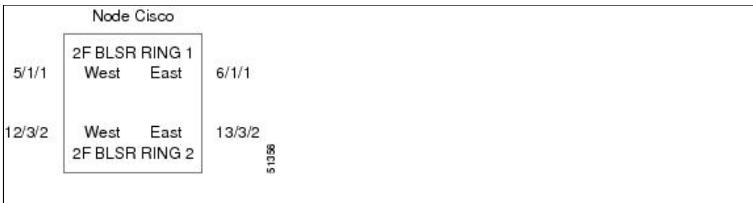
Figure 2-28: Two-Fiber BLSR to Two-Fiber BLSR
