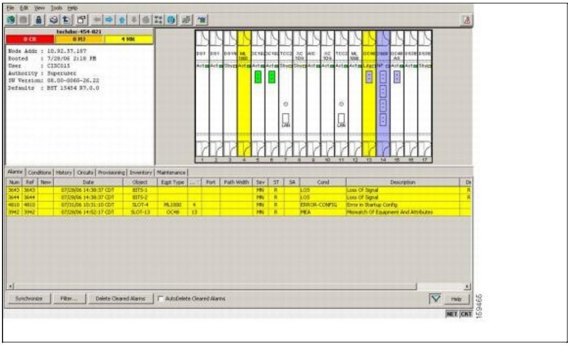
3. Use the IP address and the total of the slot number plus 2000 as the Telnet address in your preferred communication program. For example, for an IP address of 10.92.57.187 and Slot 13, you would enter or telnet <10.92.57.187 2013.>
