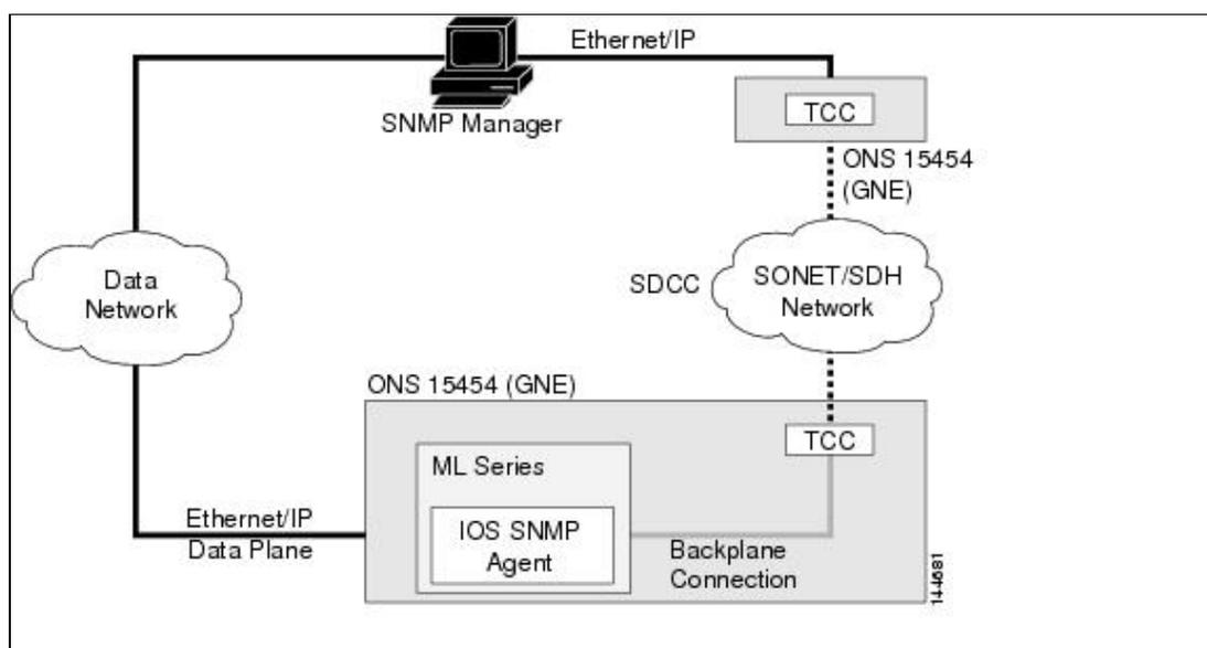
When the ONS 15454 SONET/SDH node relays the ML-Series card SNMP communication, the node uses a proxy agent to accept, validate, and forward get, getNext, and set requests to the ML-Series card. These ML-Series card requests contain the slot identification of the ML-Series card cards to distinguish the request from a general SNMP request for the ONS 15454 SONET/SDH node. The responses from the ML-Series card are then relayed by the ONS 15454 SONET/SDH node to the requesting SNMP agents.
