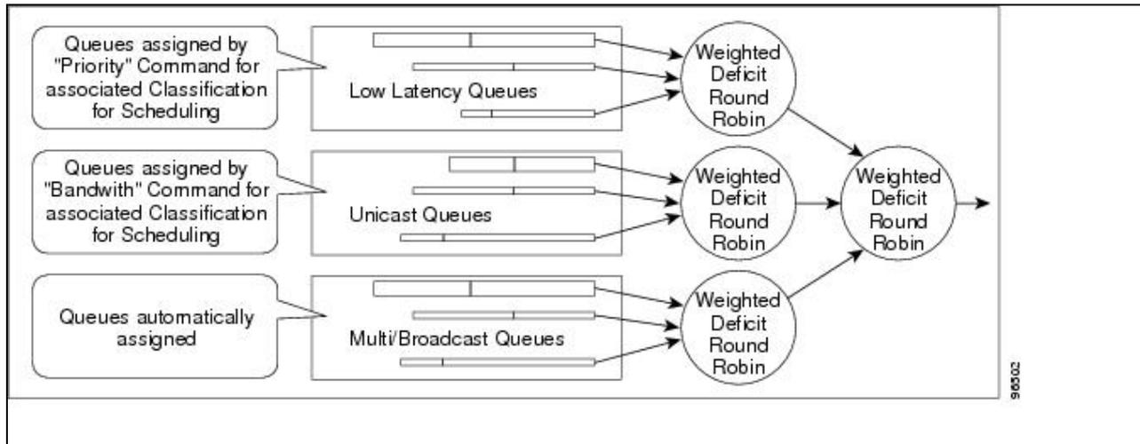
The weighting structure allows traffic to be scheduled at 1/2048 of the port rate. This equates to approximately 488 kbps for traffic exiting a Gigabit Ethernet port, approximately 293 kbps for traffic exiting an OC-12c port, and approximately 49 kbps for traffic exiting a FastEthernet port.
