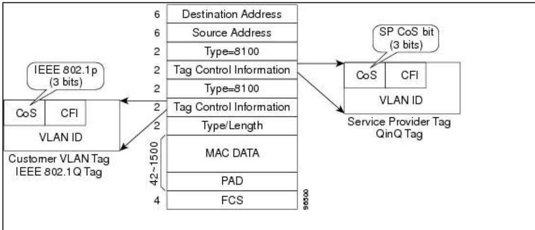
The ML-Series cards can be used as the IEEE 802.1Q tunneling device for the QinQ network and also provide the option to copy the customer frame's CoS bit into the CoS bit of the added QinQ tag. This way, the service provider QinQ network can be fully aware of the necessary QoS treatment for each individual customer frame.
