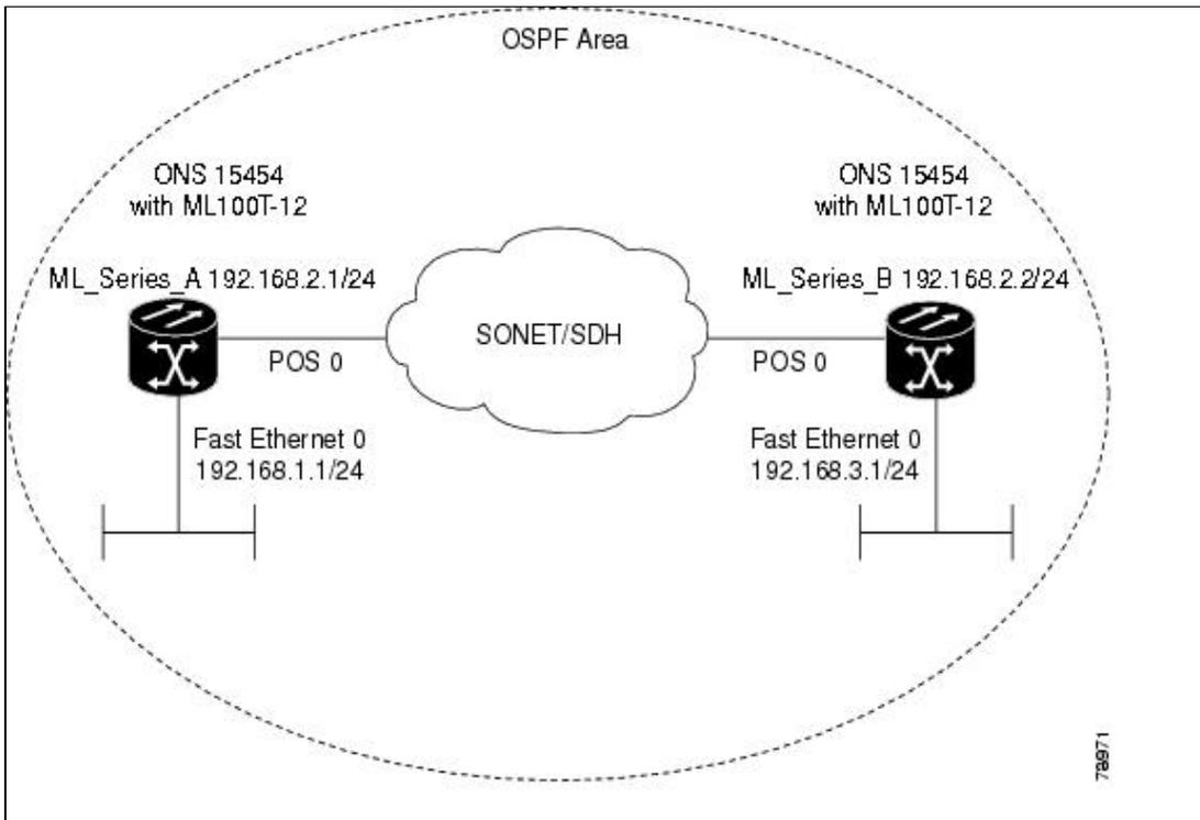
Enabling OSPF requires that you create an OSPF routing process, specify the range of IP addresses to be associated with the routing process, and assign area IDs to be associated with that range.
