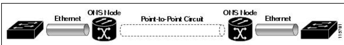
Figure 21-4: CE-100T-8 Point-to-Point Circuit
