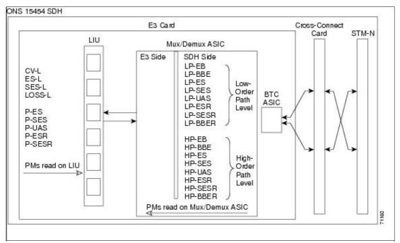
The PM parameters for the E3-12 card are listed in <u>Table 15-5</u>. The parameters are defined in <u>Table 15-5</u>.
