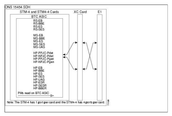
The PM parameters for the STM-4 cards are described in <u>Table 15-19</u>. The parameters are defined in <u>Table 15-3</u>.
