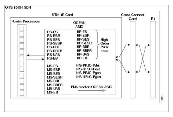
Ports 9 to 12 can be provisioned as E4 framed from the Provisioning > Ports tabs. <u>Figure 15-10</u> shows the VC4 performance monitoring parameters in E4 mode.
