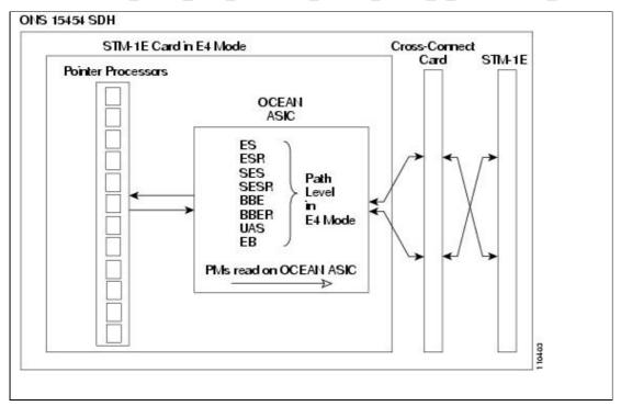
The PM parameters for the STM-1E cards are listed in <u>Table 15-18</u>. The parameters are defined in <u>Table 15-3</u>.
