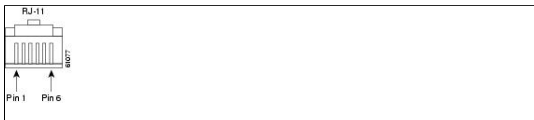
Figure 2-10: RJ-11 Cable Connector
