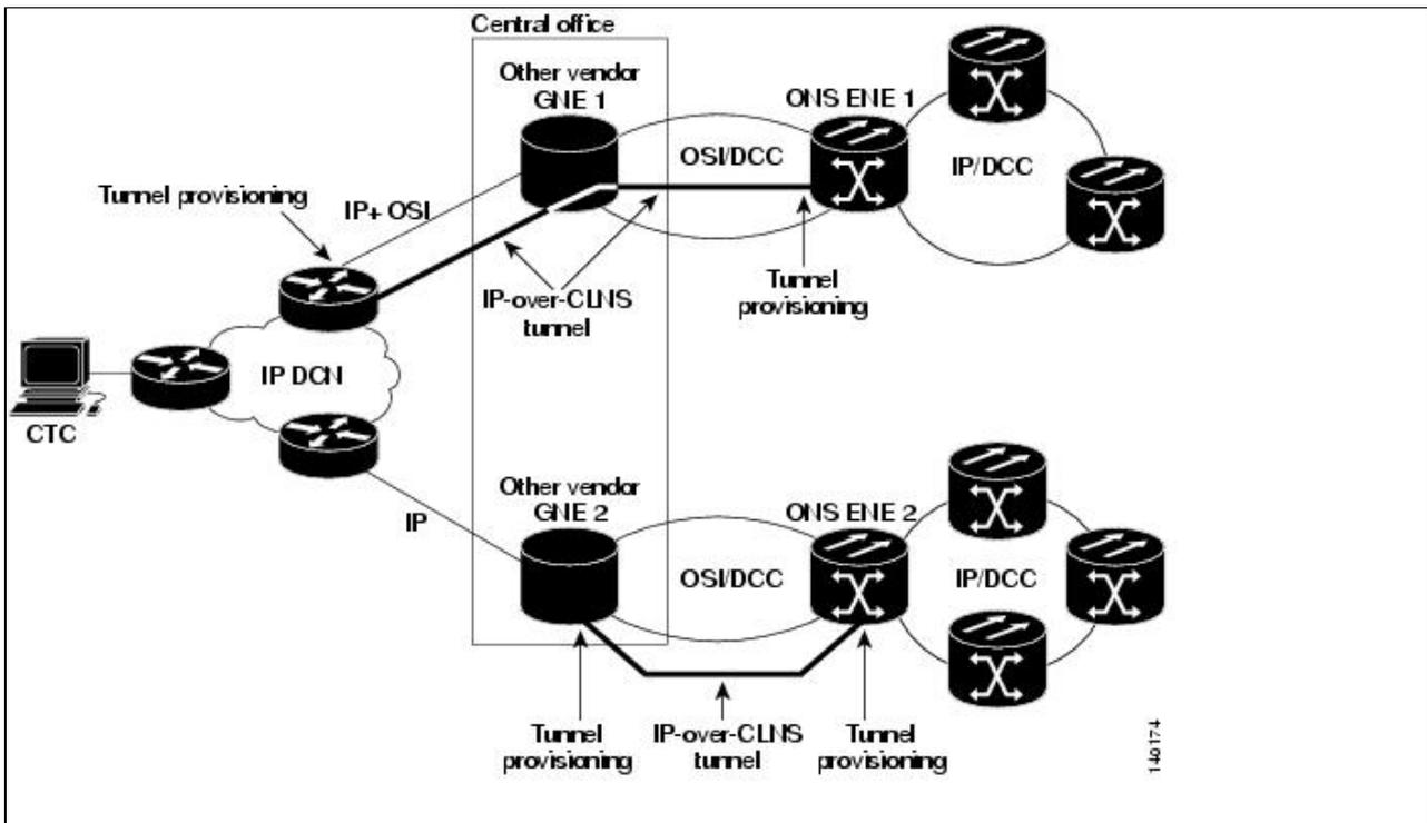
Figure 8-9 shows the same network using TL1 tunnels. Tunnel provisioning occurs at the CTC computer when the tunnel is created with the CTC Launcher. No provisioning is needed at ONS NEs, GNEs or routers.
