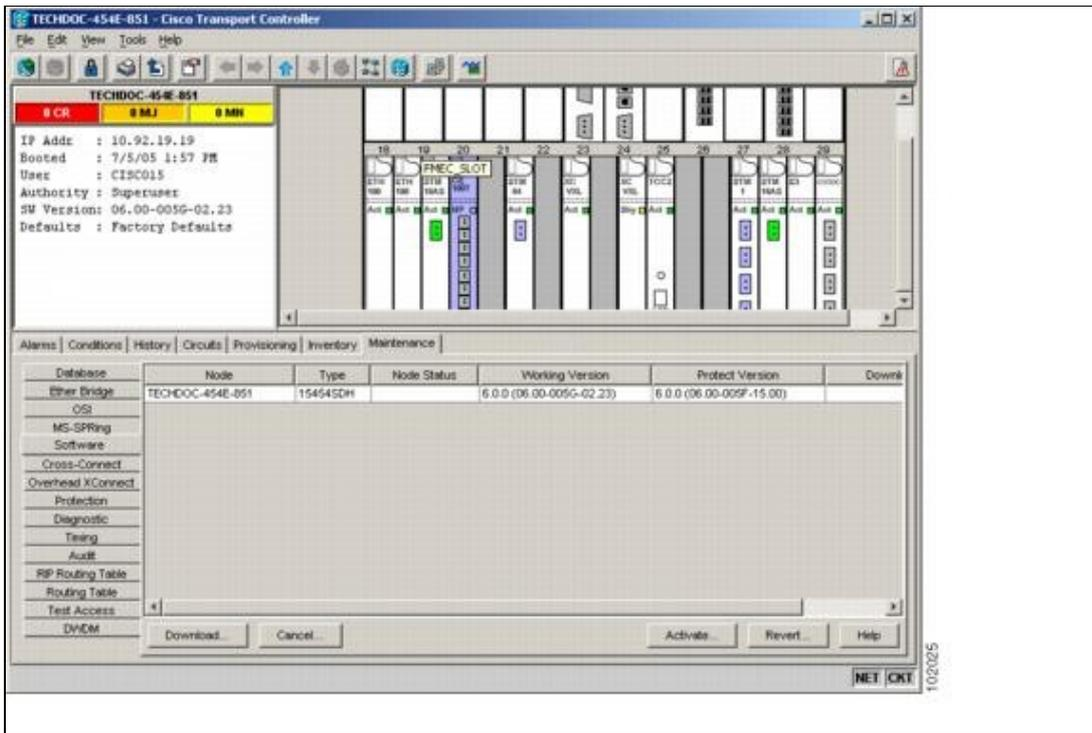
Select the Maintenance > Software tabs in network view to display the software versions installed on all the network nodes (Figure 8-2).
