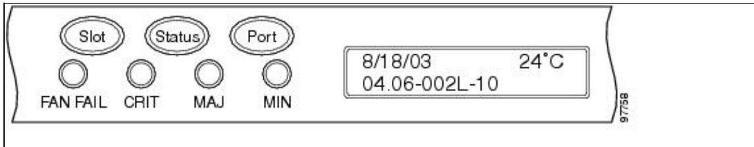
To return to the previous view from the Port screen, continue to press **Port** until the display cycles through all the ports on the slot. For instance, on the STM-3 card, press Port until it cycles past Slot 4 and you see "Slot."
