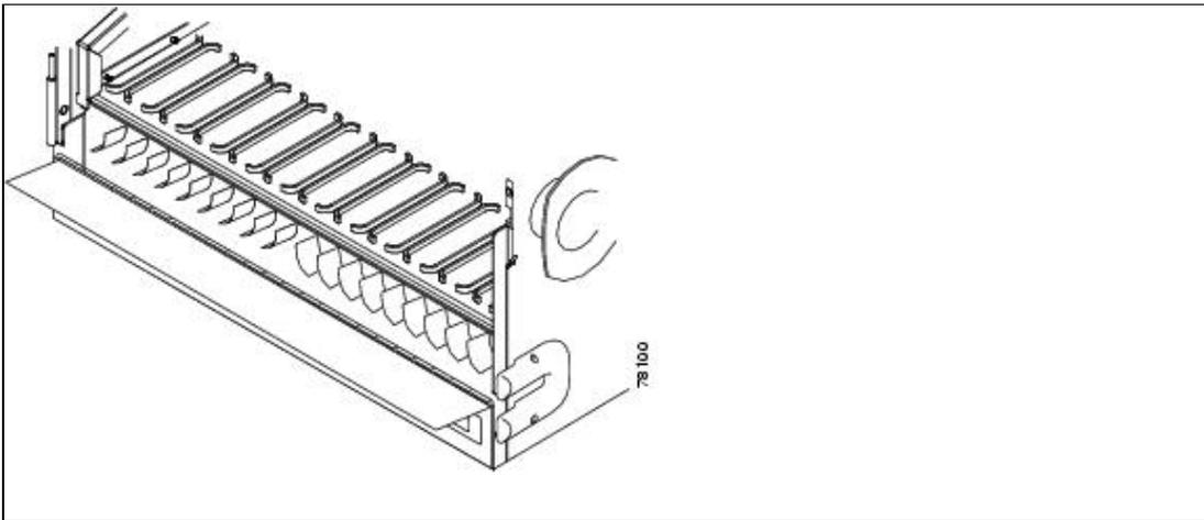
3. Route the fiber cable on the card faceplate through the fiber clip on the faceplate ([Figure 2-3](#)). Fiber clips are factory-attached to the faceplate of the STM-N cards.
