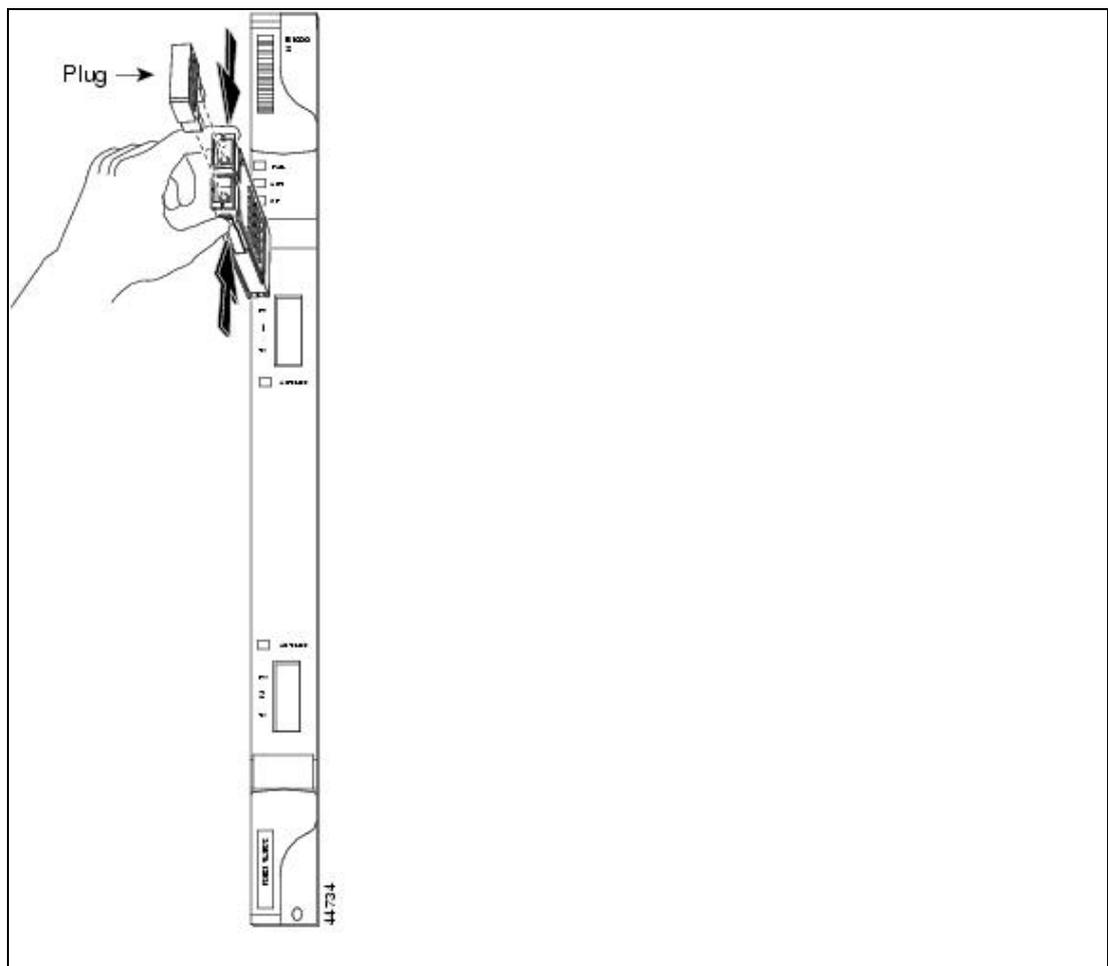
2. Slide the GBIC through the flap that covers the opening until you hear a click. The click indicates that the GBIC is locked into the slot.
