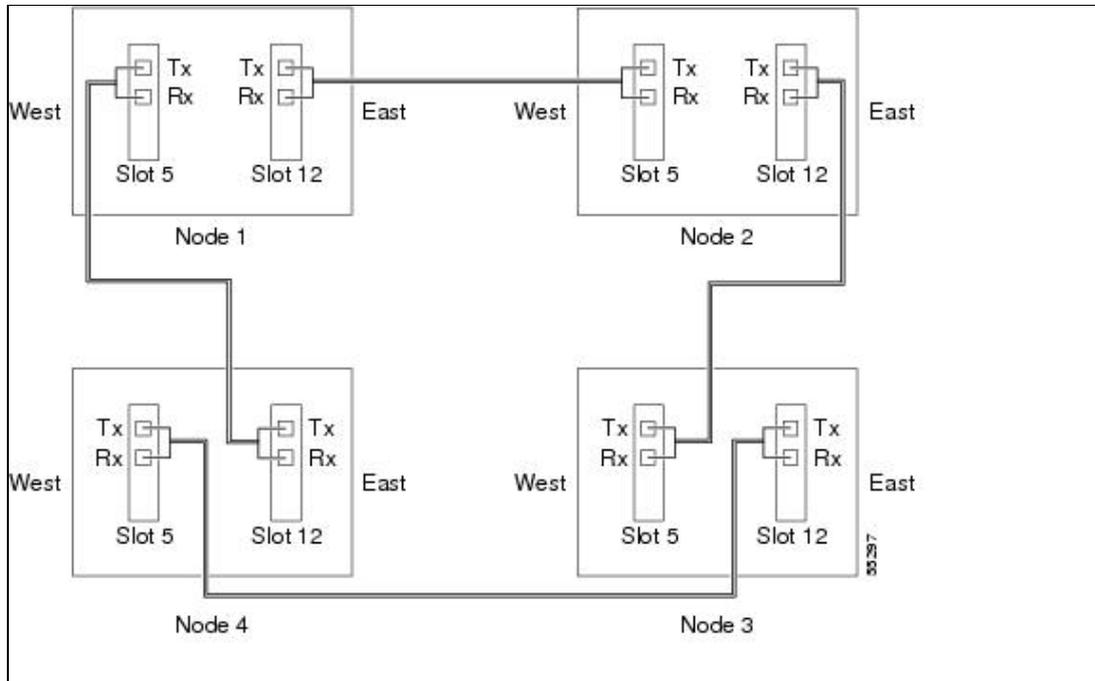
[Figure 20-10](#) shows fiber connections for a four-fiber MS-SPRing. Slot 5 (west) and Slot 12 (east) carry the working traffic. Slot 6 (west) and Slot 13 (east) carry the protect traffic.
