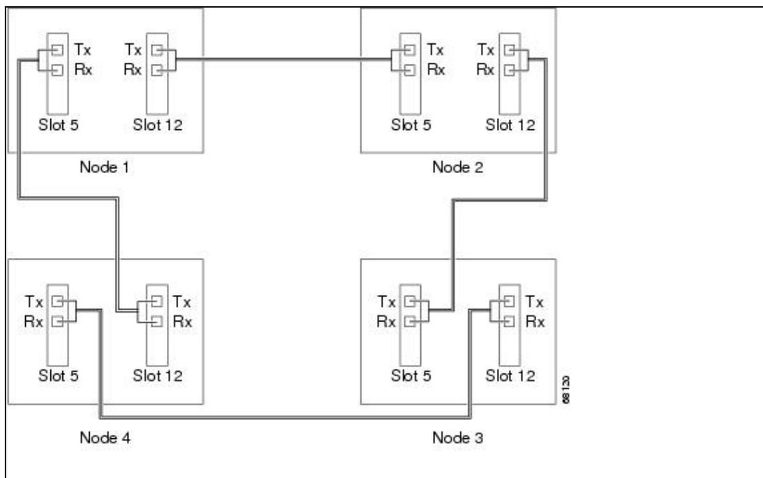
[Figure 20-7](#) shows an SNCP dual-ring interconnect (DRI) example.
