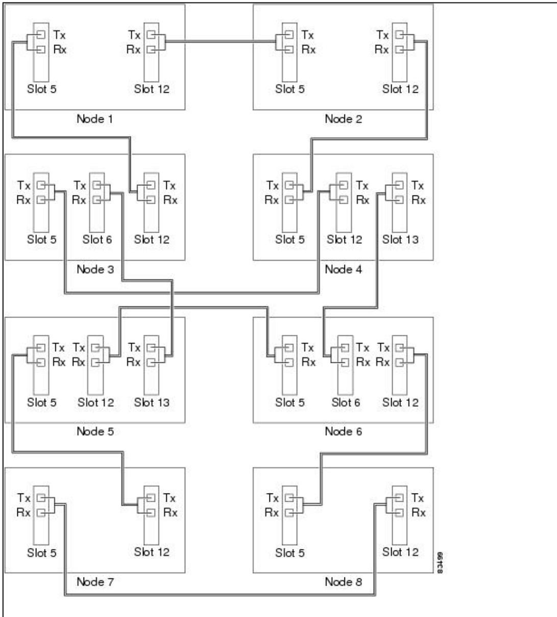
Figure 20-8 shows an integrated SNCP DRI example.
