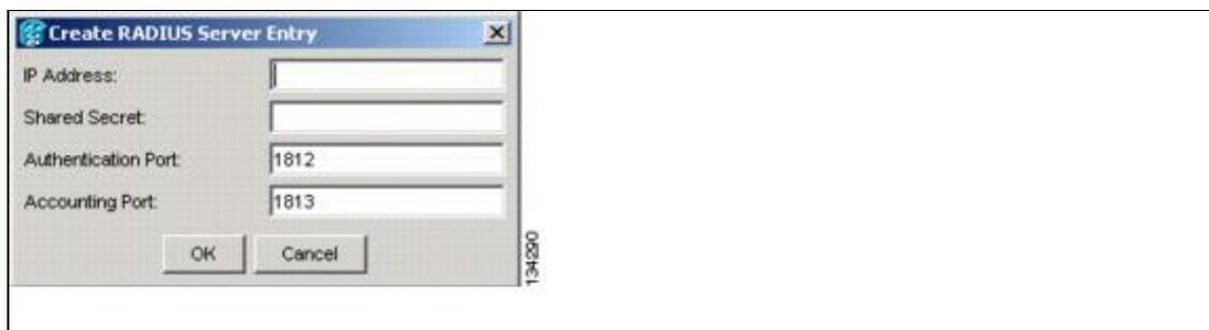
3. Enter the RADIUS server IP address in the IP Address field. If the node is an end network element (ENE), enter the IP address of the gateway network element (GNE) in this field.
