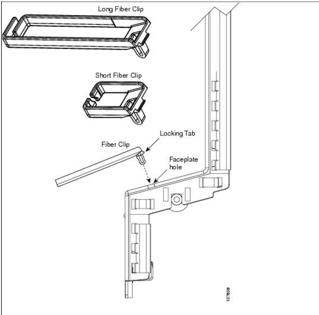
3. Push the clip into the hole until the locking tab snaps the clip securely into place. To remove a fiber clip, push on the locking tab to release the clip while rotating the clip forward and up.
