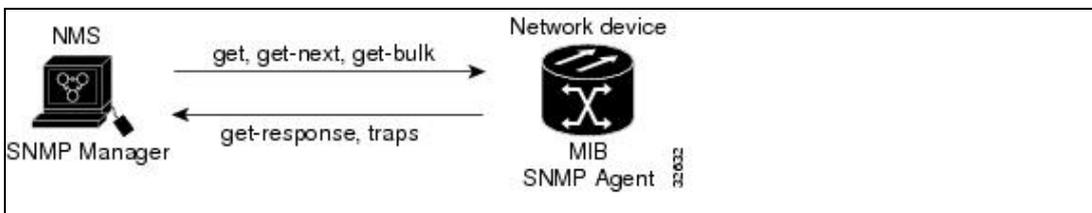
The SNMP agent captures data from MIBs, which are device parameter and network data repositories, or from error or change traps.
