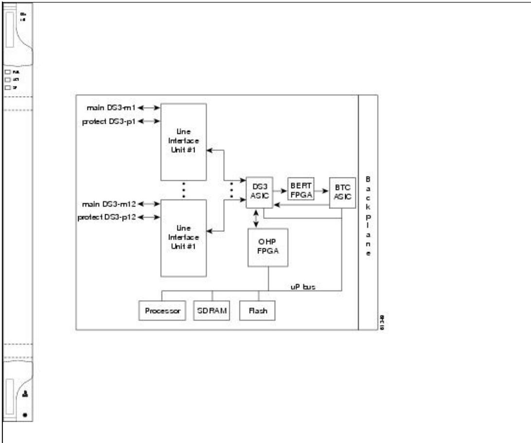
[Figure 3-10](#) shows the DS3N-12E faceplate and a block diagram of the card.
