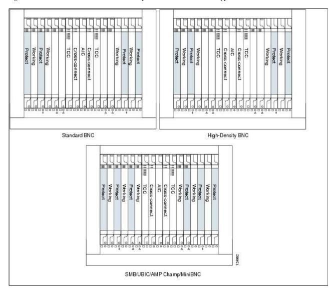
Figure 7-4: Unprotected High-Density Electrical Card Schemes for EIA Types
