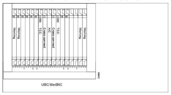
Figure 7-5 shows 1:1 low-density card protection by EIA type.
