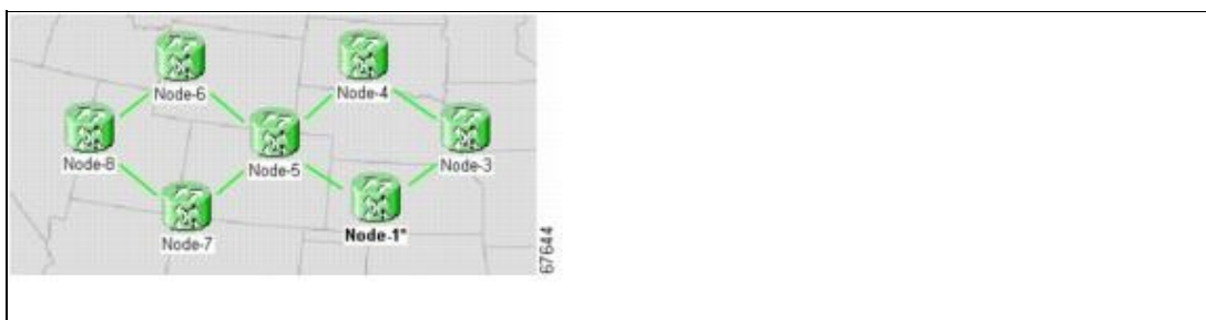
Figure 5-14: Subtended BLSRs on the Network Map
