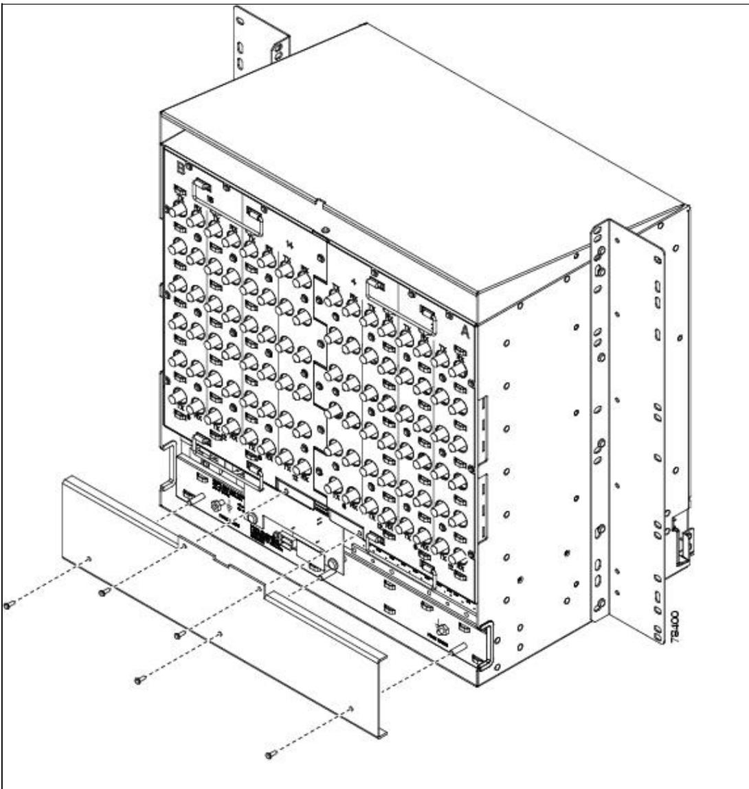
5. Tighten the five retaining screws that hold the plastic cover in place.
