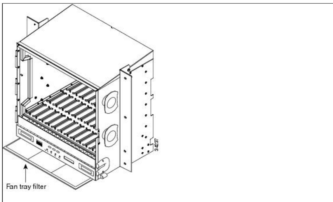
5. Push the outer side of the handles on the fan-tray assembly to expose the handles.
