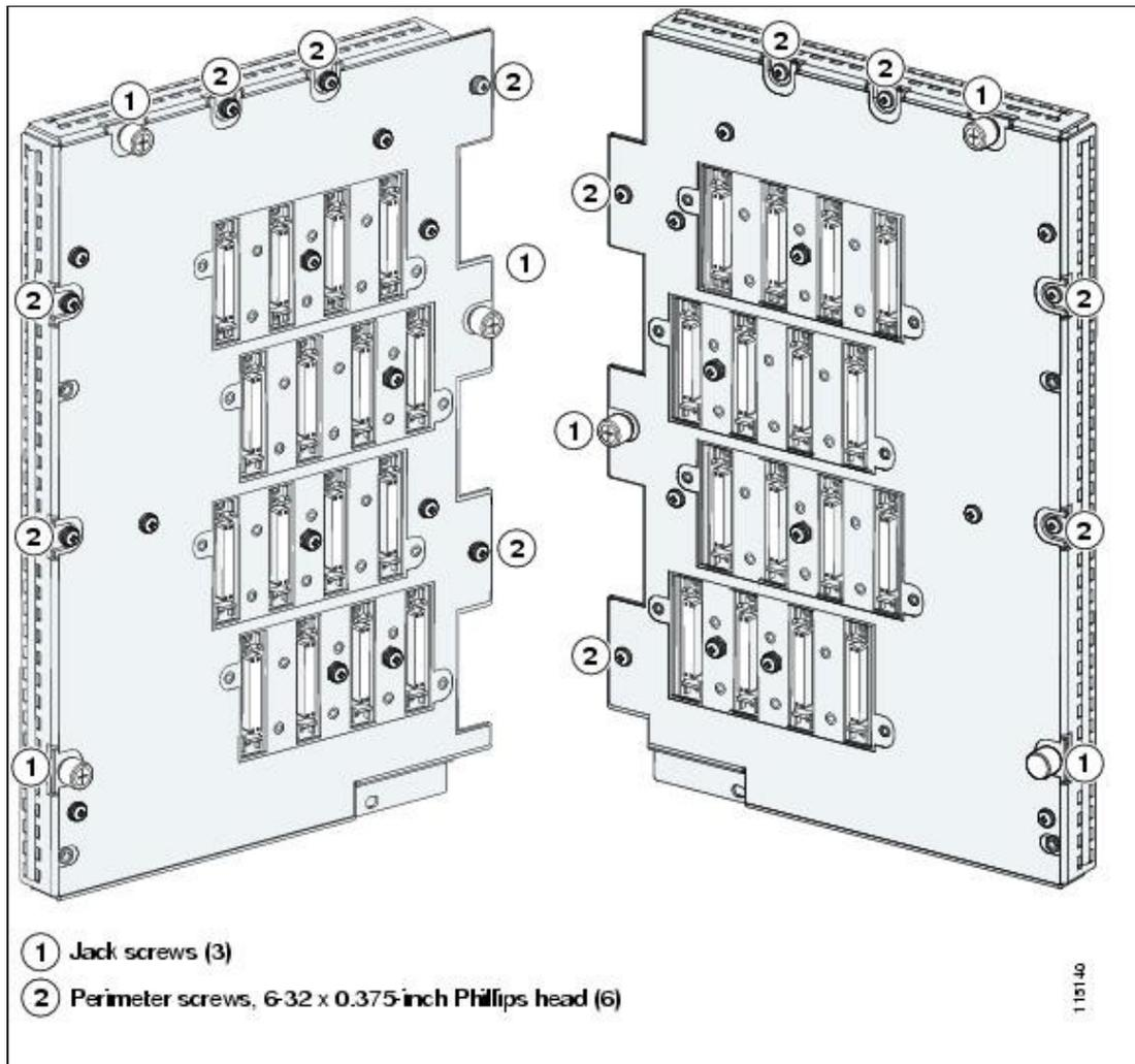
3. Use a Phillips screwdriver to loosen each jack screw a maximum of two turns. Rotate each jack screw two turns at a time (per the rotation indicator) until all jack screws are fully disengaged ([Figure 15-14](#)).
