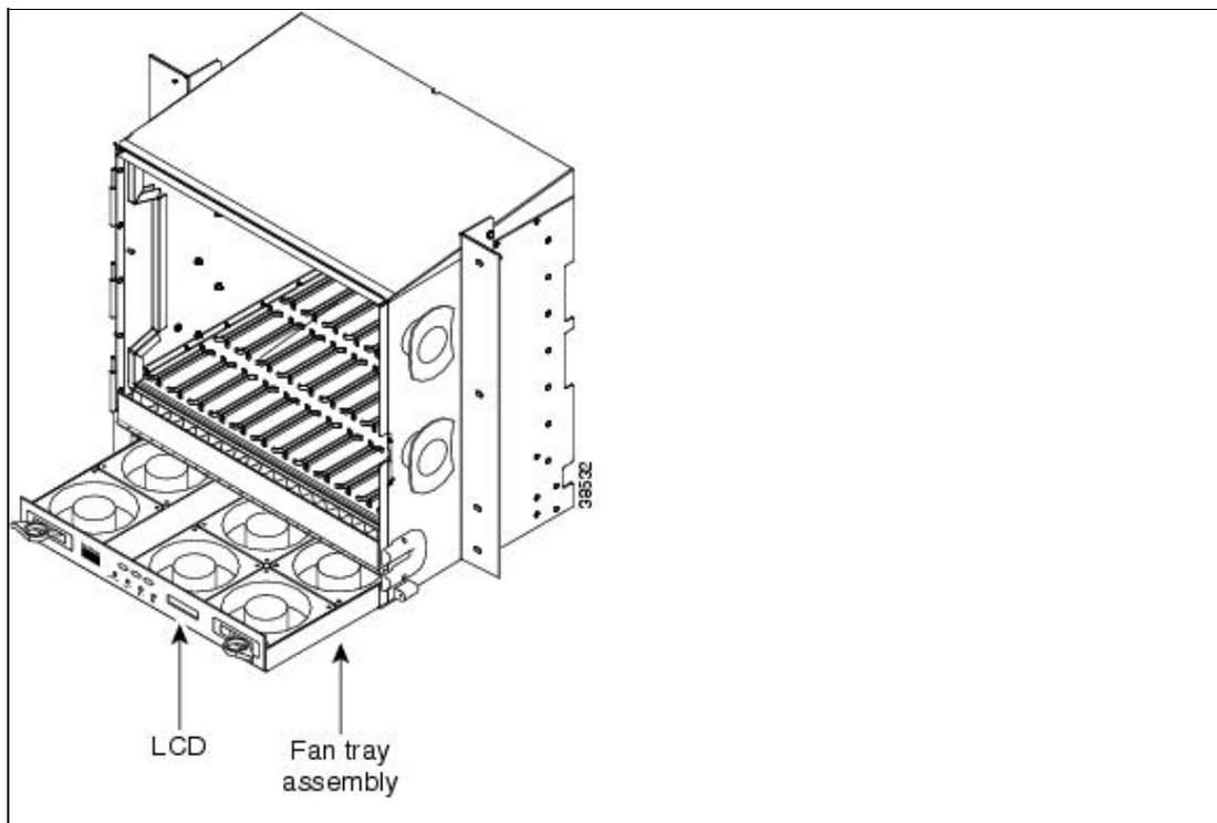
8. If you are replacing the fan-tray air filter and it is installed beneath the fan-tray assembly, slide the existing air filter out of the shelf assembly and replace it before replacing the fan-tray assembly.
