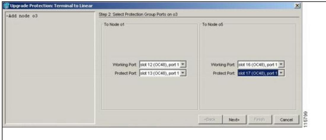
8. Select the working and protect ports on the new node in the drop-down lists that you want to connect to each terminal node.
