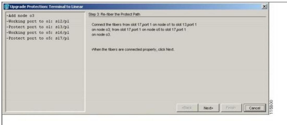
10. Follow the instructions in the Re-fiber the Protected Path dialog box for connecting the fibers between the nodes.
