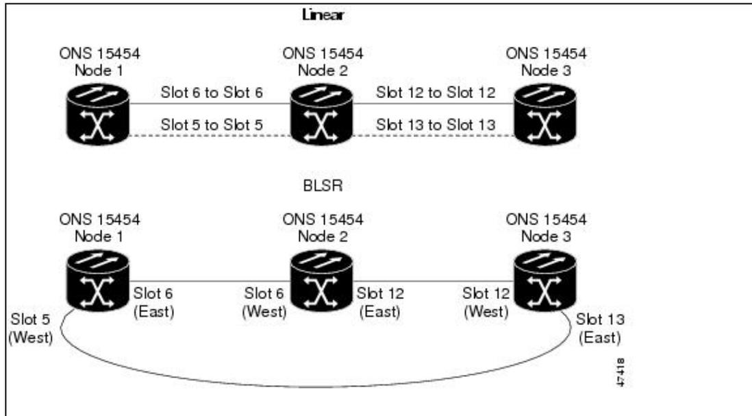
10. Create the ring by connecting the protect fiber from one end node to the protect port on the other end node. For example, the fiber between Node 1/Slot 5 and Node 2/Slot 5 (as shown in [Figure 13-3](#)) can be rerouted to connect Node 1/Slot 5 to Node 3/Slot 13.
