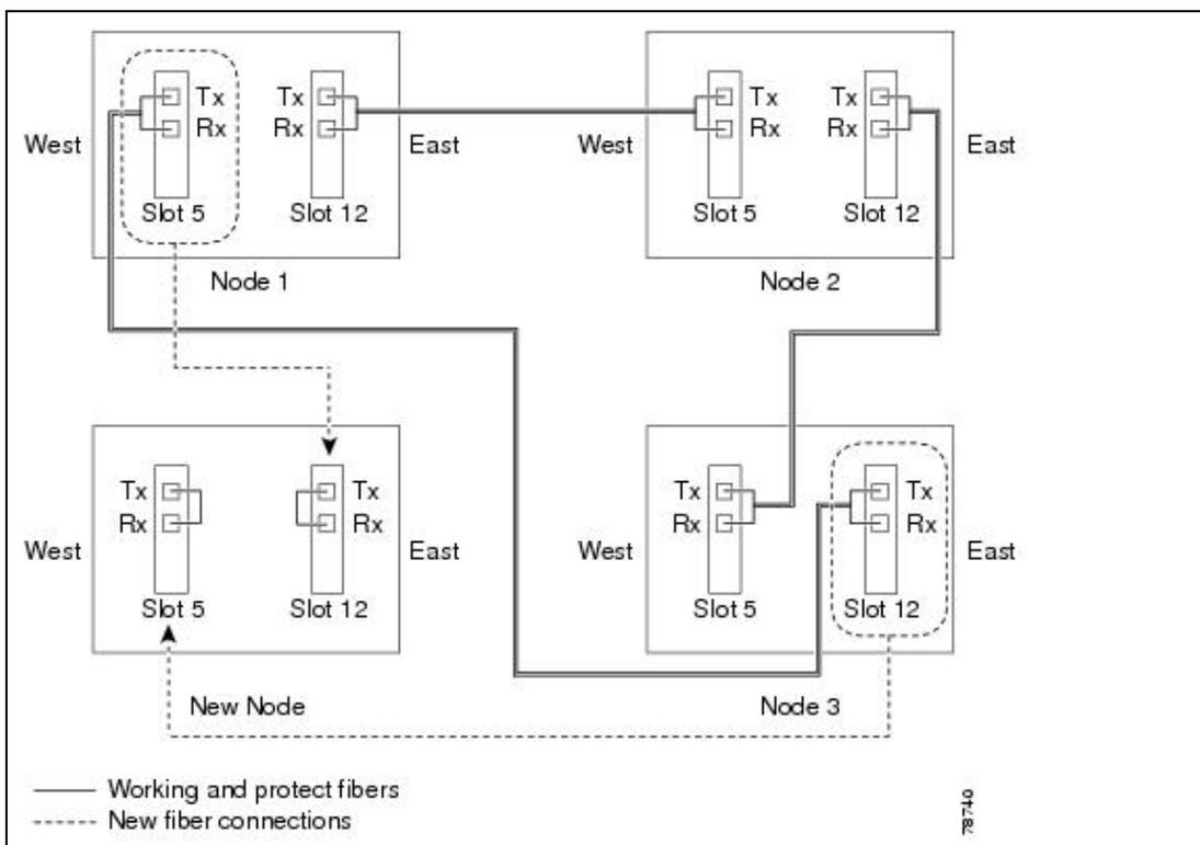
[Figure 14-2](#) shows a sample drawing of a three-node, four-fiber BLSR. The dashed arrow shows the new fiber connections that will be made to add the fourth node. For four-fiber BLSRs, two fiber sets will be reconnected, the working fiber and the protect fiber.
