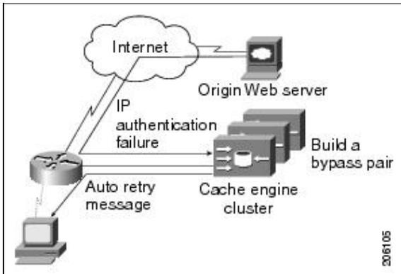
In Figure: Dynamic Client Bypass, when the client's browser automatically issues a reload, the request will be redirected to the cache engine. However, when the bypass table is checked and the request matches one of the table entries, the cache engine will refuse the request and send it directly to the origin Web server. Thus, the origin Web server will see the client's IP address, authenticate the client, and respond directly to the client.
