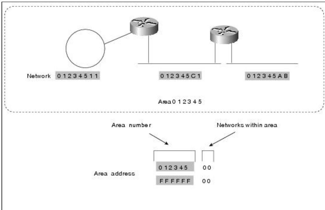
A routing area can have as many as three different area addresses, each with a different mask. Having more than one area address allows the routing area to be reorganized without interrupting operations. Any combination of area addresses can be used within a domain.
