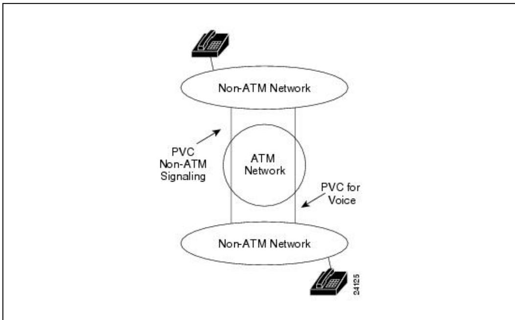
At no time is the ATM network participating in the interpretation of the signaling that takes place between end stations. However, as a value-added feature, some products are capable of understanding channel associated signaling (CAS) and can prevent the sending of empty voice cells when the end stations are on-hook.
