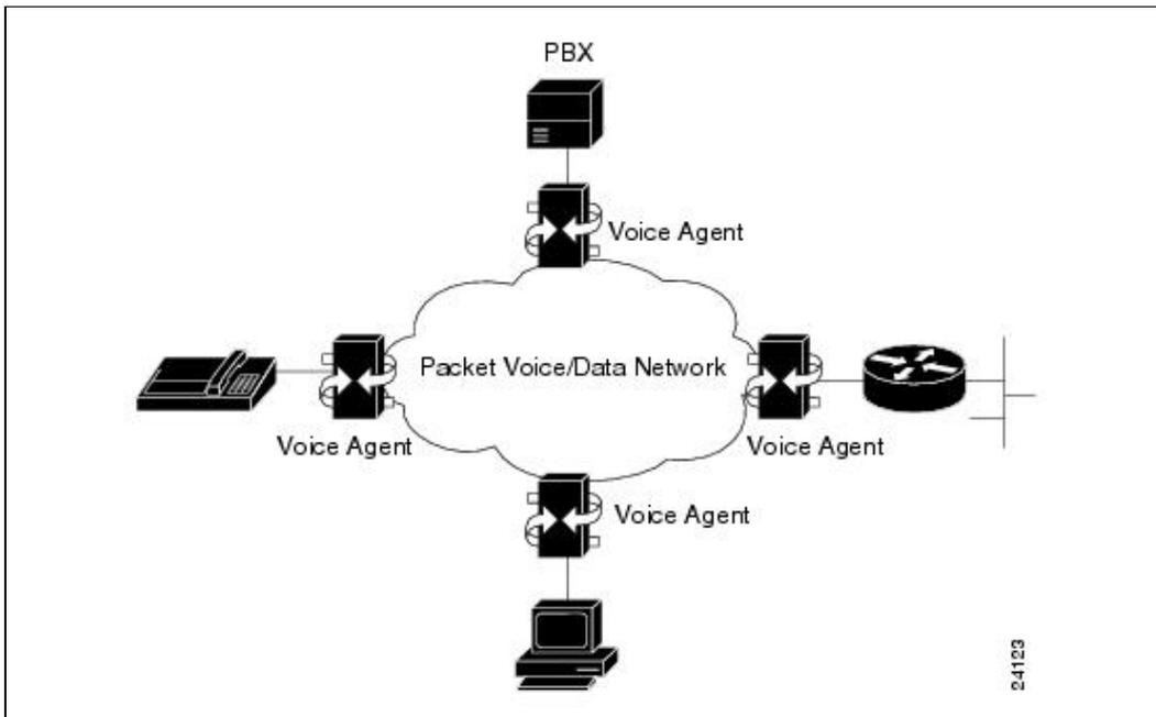
This voice agent connection model shows that there are two issues in packet voice networking that must be explored to ensure that packet voice services meet user needs. The first issue is voice coding-how voice information is transformed into packets, and how the packets are used to re-create the voice. Another issue is the signaling associated with identifying who the calling party is trying to call and where the called party is in the network.
