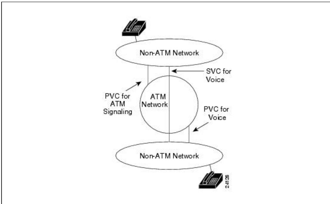
A signaling request from an end station causes the ATM network to create an SVC with the appropriate QoS to the desired end station. The creation of an SVC versus the prior establishment of PVCs is clearly more advantageous for three reasons:
