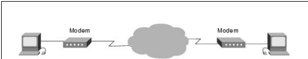
Figure: A Modem Connection Through a WAN Handles Analog and Digital Signals
