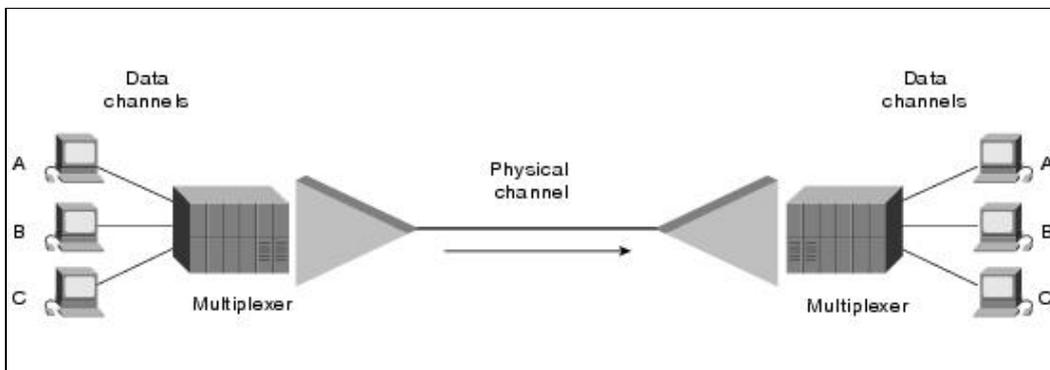
A multiplexer is a physical layer device that combines multiple data streams into one or more output channels at the source. Multiplexers demultiplex the channels into multiple data streams at the remote end and thus maximize the use of the bandwidth of the physical medium by enabling it to be shared by multiple traffic sources.
