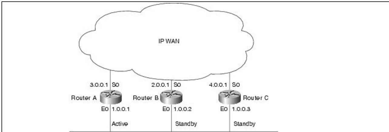
In Figure: A network with tracking configured, Router A is configured as the active router. Routers B and C are configured as standby routers for Router A. The following is the configuration for Router A:
