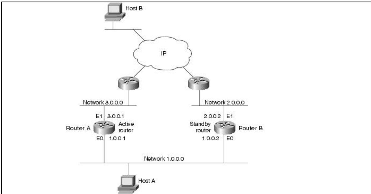
All hosts on the network are configured to use the IP address of the virtual router (in this case, 1.0.0.3) as the default gateway. The command for configuring the default gateway depends on the host's operating system, TCP/IP implementation, and configuration.
