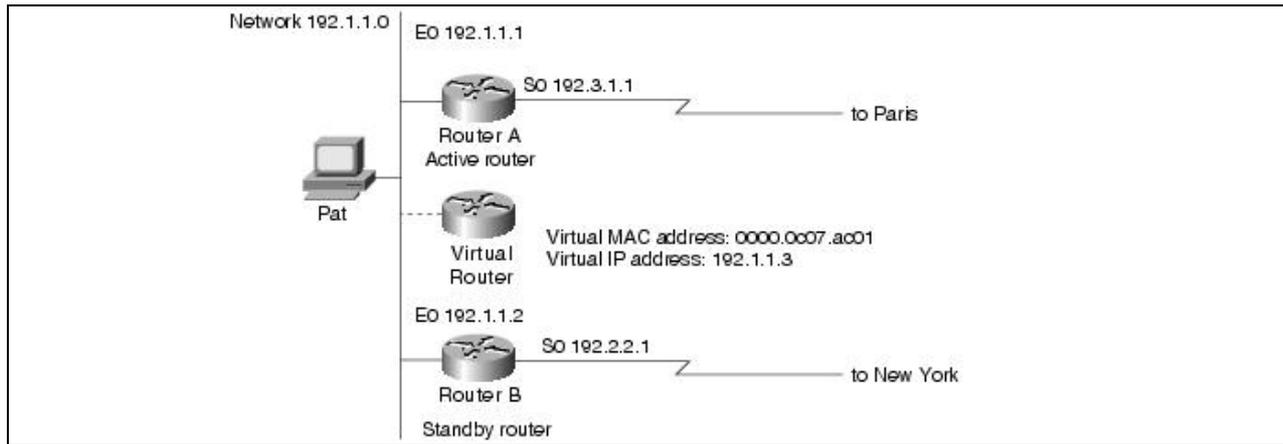
In Figure: HSRP addressing on the Tokyo segment, the MAC address of the virtual router is 0000.0c07.ac01. When you configure HSRP, the router automatically selects one of the virtual MAC addresses from a range of addresses in the Cisco IOS software that is within the range of Cisco's MAC address block. Ethernet and FDDI LANs use one of the preassigned MAC addresses as a virtual MAC address. Token Ring LANs use a functional address as a virtual MAC address.
