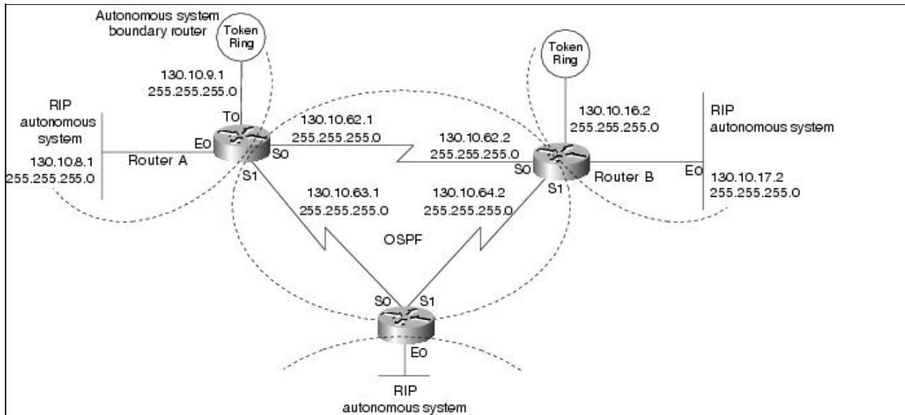
RIP does not need to run between the backbone routers; therefore, RIP is suppressed on Router A with the following commands:
