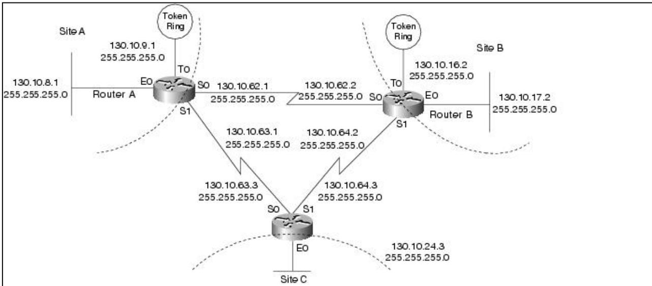
Table: RIP Network Address Assignments lists the network address assignments for the RIP network, including the network number, subnet range, and subnet masks. All interfaces indicate network 130.10.0.0; however, the specific address includes the subnet and subnet mask. For example, serial interface 0 on Router C has an IP address of 130.10.63.3 with a subnet mask of 255.255.255.0.
