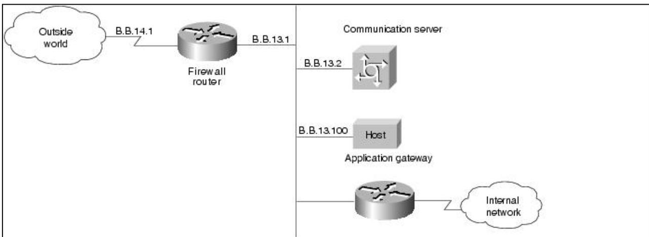
In this case study, the firewall router allows incoming new connections to one or more communication servers or hosts. Having a designated router act as a firewall is desirable because it clearly identifies the router's purpose as the external gateway and avoids encumbering other routers with this task. In the event that the internal network needs to isolate itself, the firewall router provides the point of isolation so that the rest of the internal network structure is not affected.
