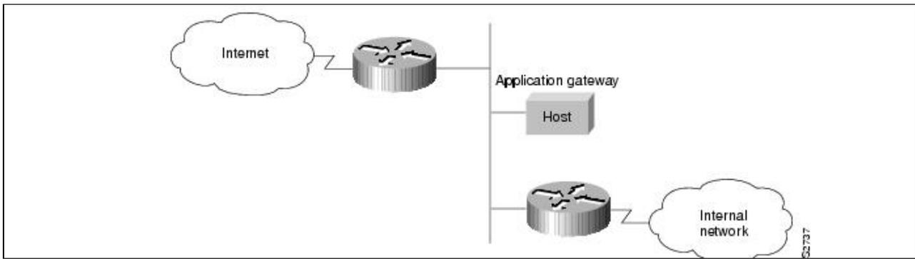
In this architecture, the router that is connected to the Internet (exterior router) forces all incoming traffic to go to the application gateway. The router that is connected to the internal network (interior router) accepts packets only from the application gateway.
