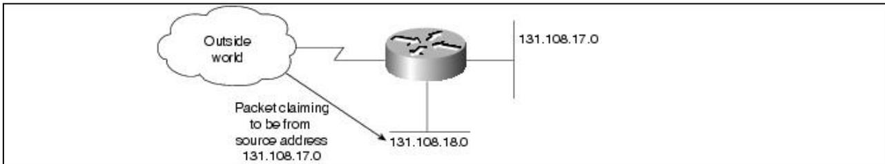
If you have several internal networks connected to the firewall router and the router is using output filters, traffic between internal networks will see a reduction in performance created by the access list filters. If input filters are used only on the interface going from the router to the outside world, internal networks will not see any reduction in performance.
