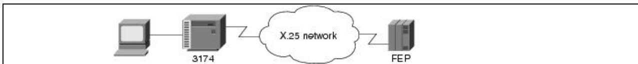
Figure: Typical QLLC topology
