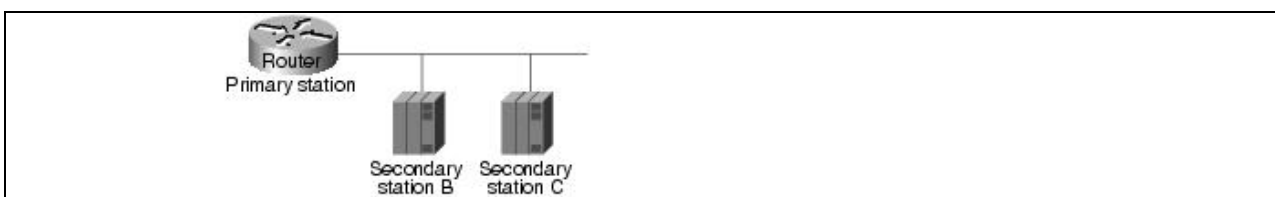
Figure: Two-way simultaneous mode in a multidrop environment
