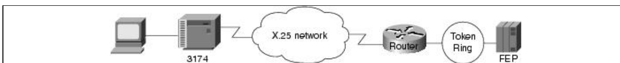
Figure: Simple topology for QLLC conversion
