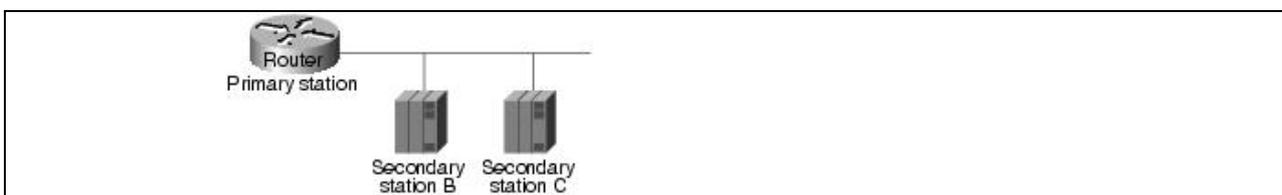
The **sdlc simultaneous** command enables two-way simultaneous mode in a multidrop environment. When two-way simultaneous mode is enabled for a point-to-point connection to a secondary station, the router can send data to the secondary station even if there is an outstanding poll, as long as the window size limit is not reached. The **sdlc simultaneous** command with the single keyword enables two-way simultaneous mode in a point-to-point link environment.
