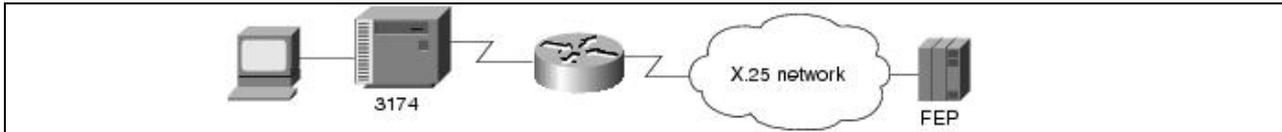
QLLC conversion also supports multiple SDLC connections coming through an MSD, as shown in [Figure: QLLC conversion supports multidrop SDLC topology](#).
