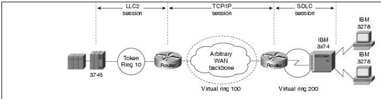
**Note:** Local acknowledgment requires that TCP sessions be maintained between the routers. It is not uncommon to see high router CPU utilization at idle traffic times and then decreased utilization as traffic increases. Polling overhead in the router may increase processor use.
