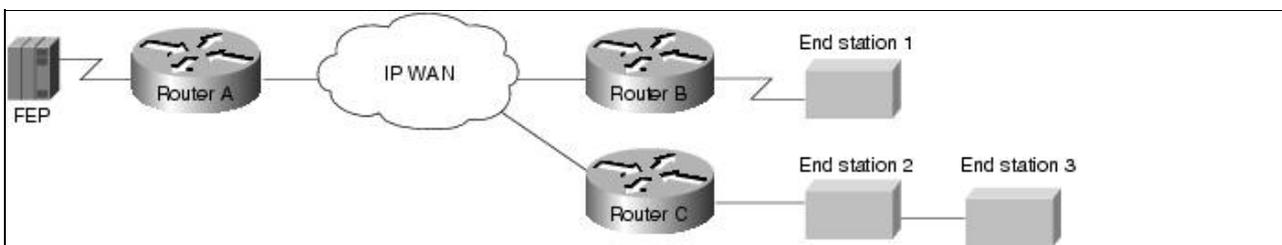
The **sdlc virtual-multidrop** interface configuration command enables SDLC broadcast and should be used only on the router that is configured as the secondary station on the SDLC link. In addition, the **stun route address tcp** command for SDLC address 0xFF must be configured on the secondary station (in this example, Router A) for each STUN peer. A sample configuration follows:
