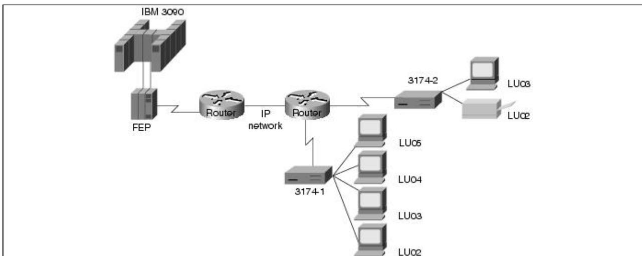
As of Software Release 9.1(9), LU address prioritization for both remote source-route bridging (RSRB) and STUN solved this problem. In addition to the LU address, you can specify the SDLC address to identify a PU in a multidropped SDLC line. The syntax of the **locaddr-priority** global configuration command follows:
