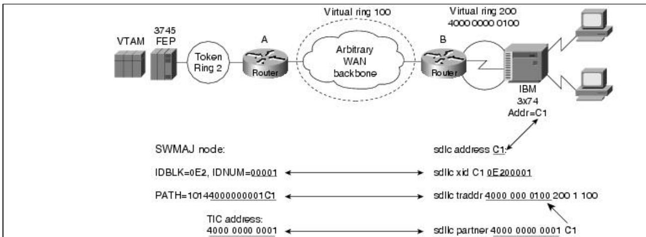
Consider an example of two routers that implement the SDLLC functionality in an environment that interconnects a remote site to a host channel attached to a 3174 Token Ring gateway, as shown in [Figure: SDLLC implementation with 3174 Token Ring gateway](#).
