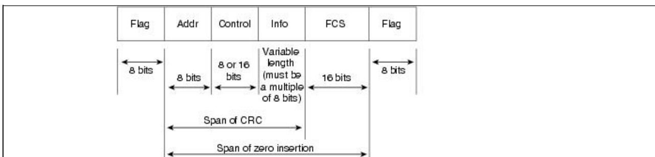
The Flag field starts and ends the frame and initiates and terminates error checking. When the link is idle, the router sends streaming flags to maintain link synchronization, but this is not necessary to keep the link up.
