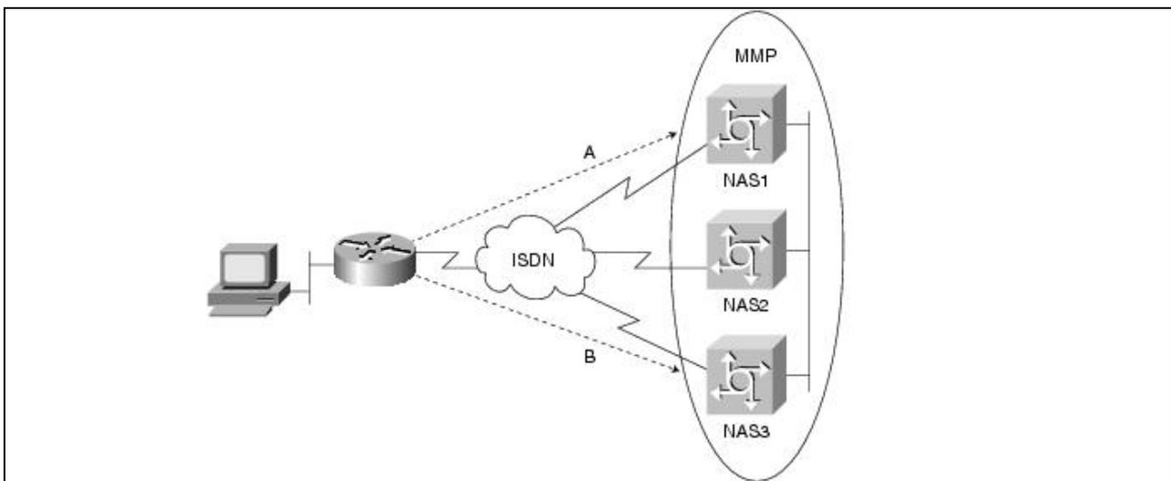
Cisco recognized that no matter what size NAS they can develop, there will always be customers needing larger pools of access ports. As such, Cisco IOS 11.2 released Multichassis MultiLink Point-to-Point Protocol (MMP), which extends MultiLink PPP (MLP) by providing a mechanism to aggregate B channels transparently across multiple NASs.
