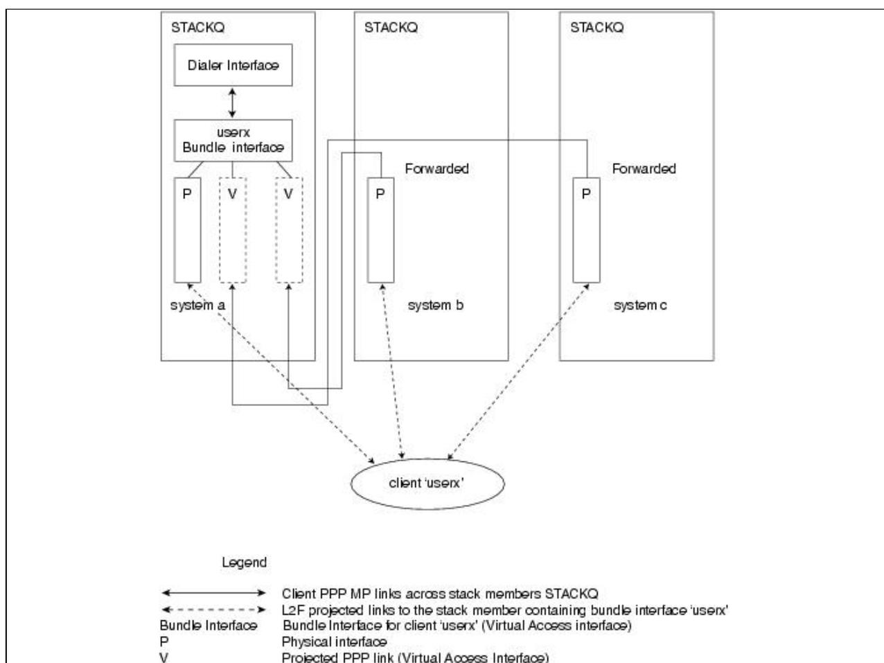
MMP provides an interoperable multivendor solution because it does not require any special software capabilities at the remote sites. The only remote requirement is support for the industry standard MLP ([RFC 1717](#)).
