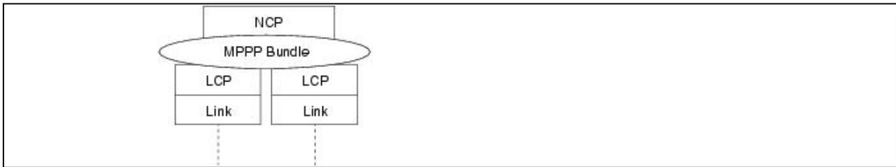
When an NCP packet arrives at an MLP master-interface for transmitting and is over 30 bytes, it is fragmented and sent on each physical link in the MLP bundle. When MLP packet fragments arrive on PPP destination, MLP reassembles the original packets and sequences them correctly in the data stream.
