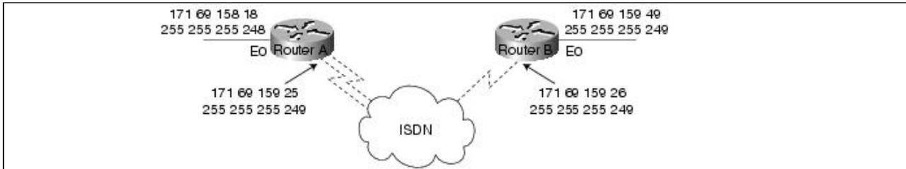
Using the configuration that follows, BRI 0 is activated only when serial interface 1/0 (the primary line) goes down. The **backup delay** command configures the backup connection to activate 30 seconds after serial interface 0 goes down and to remain activated for 60 seconds after the serial interface 1/0 comes up:
