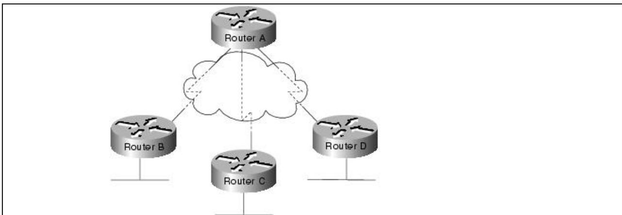
Hub-and-spoke topologies are easier to configure than fully meshed topologies when multipoint topologies are required because remote site dialer interfaces are mapped only to the central site. This allows most of the design complexity (such as addressing, routing, and authentication) to be managed on the DDR Hub. Configuration support of the remote sites can be greatly simplified (similar to one end of a point-to-point topology).
