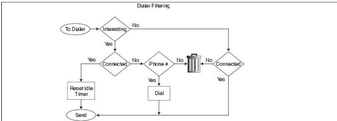
Each packet arriving at a dialer interface is filtered and determined to be interesting or uninteresting based on **dialer-group** and **dialer-list** configuration. The following Cisco IOS configuration interface dialer 1 uses dialer-group 5 to determine interesting packets, as defined by the dialer-list 5 commands. Dialer-group 5 is defined by dialer-list 5 commands which in this case deems all IP, IPX, and AppleTalk packets to be interesting.
