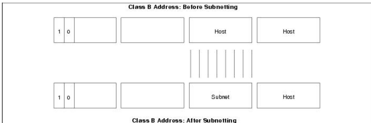
Subnet masks use the same format and representation technique as IP addresses. The subnet mask, however, has binary 1s in all bits specifying the network and subnetwork fields, and binary 0s in all bits specifying the host field.
