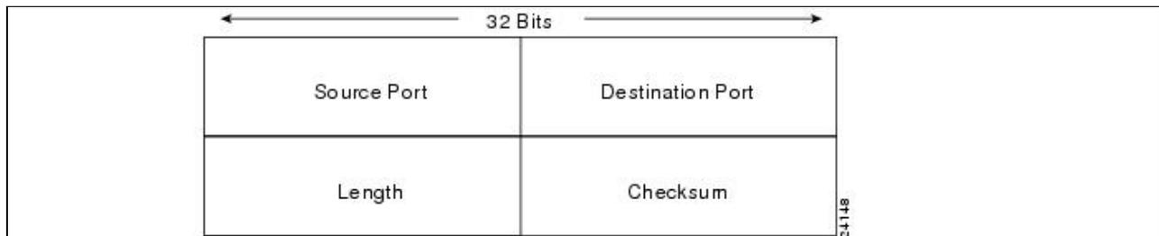
Source and destination ports contain the 16-bit UDP protocol port numbers used to demultiplex datagrams for receiving application-layer processes. A length field specifies the length of the UDP header and data. Checksum provides an (optional) integrity check on the UDP header and data.
