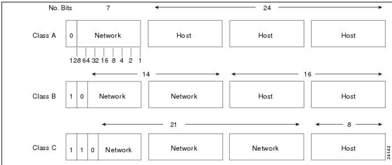
The class of address can be determined easily by examining the first octet of the address and mapping that value to a class range in the following table. In an IP address of 172.31.1.2, for example, the first octet is 172. Because 172 falls between 128 and 191, 172.31.1.2 is a Class B address.
