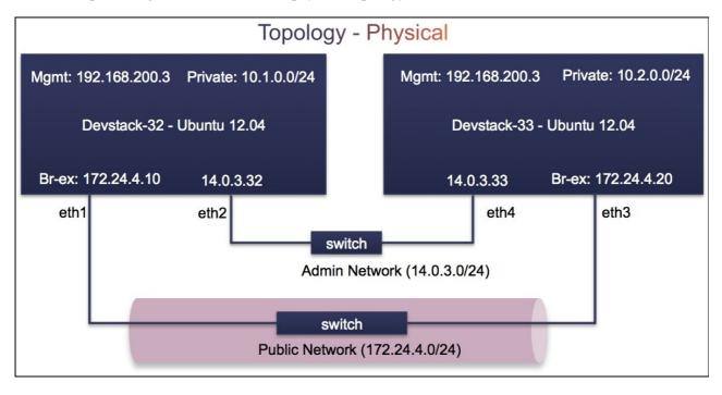
There are two UCS systems, which will each host an OpenStack (using DevStack) cloud for the site-to-site VPN end-points. A physical connection between the two nodes will be used for the "public" network (172.24.4.0/24), where traffic between the private networks (10.1.0.0/24 and 10.2.0.0/24) will be encrypted. There is an internal network on the node (192.168.200.0/24) for management of the CSR during operation, and another network (14.0.3.0/24) for setup of the clouds.
