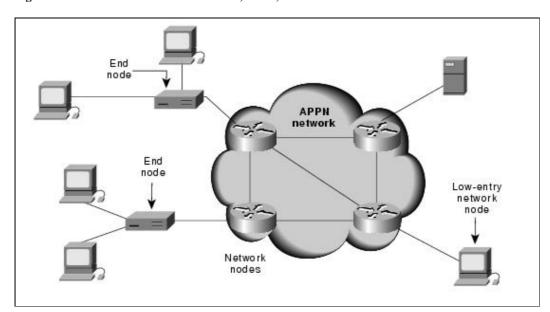
Figure: APPN Network Nodes Link to ENs, LENs, and Other Network Nodes
