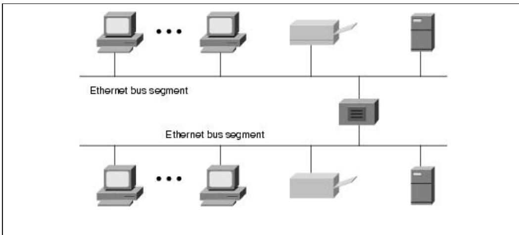
Although new networks are no longer connected in a bus configuration, some older bus-connected networks do still exist and are still useful.
