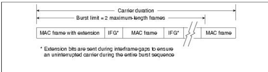
If the length of the first frame is less than the minimum frame length, an extension field is added to extend the frame length to the value indicated in [Table: Limits for Half-Duplex Operation](#). Subsequent frames in a frame-burst sequence do not need extension fields, and a frame burst may continue as long as the burst limit has not been reached. If the burst limit is reached after a frame transmission has begun, transmission is allowed to continue until that entire frame has been sent.
