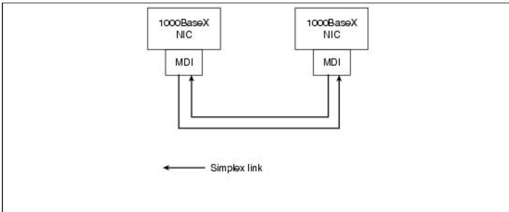
The principal differences among the 1000Base-X versions are the link media and connectors that the particular versions will support and, in the case of optical media, the wavelength of the optical signal (see [Table: 1000Base-X Link Configuration Support](#)).
