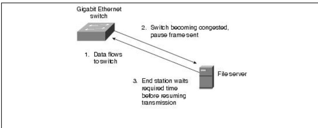
The full-duplex operation and its companion flow control capability are both options for all Ethernet MACs and all transmission rates. Both options are enabled on a link-by-link basis, assuming that the associated physical layers are also capable of supporting full-duplex operation.
