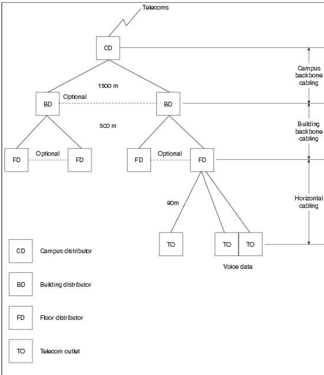
The ISO/IEC 11801 cable model is the network model on which the IEEE 802.3 standards are based:
