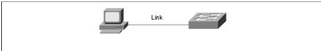
Figure: Example Point-to-Point Interconnection
