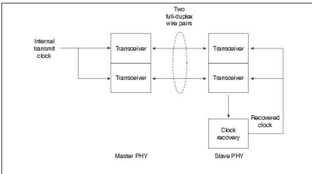
**Figure: The 100Base-T2 Link Topology**
