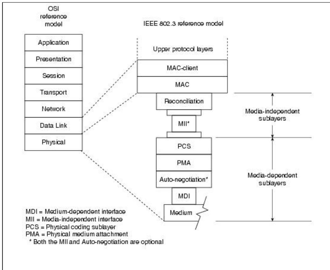
The physical layer for each transmission rate is divided into sublayers that are independent of the particular media type and sublayers that are specific to the media type or signal encoding.
