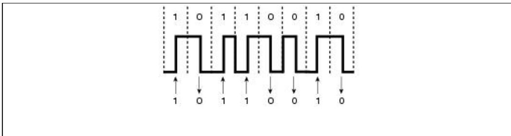
Unfortunately, Manchester encoding introduces some difficult frequency-related problems that make it unsuitable for use at higher data rates. Ethernet versions subsequent to 10Base-T all use different encoding procedures that include some or all of the following techniques:
