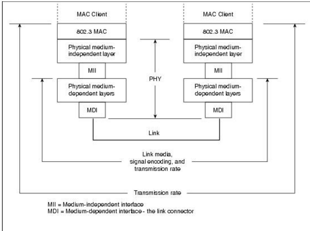
The MAC layer controls the node's access to the network media and is specific to the individual protocol. All IEEE 802.3 MACs must meet the same basic set of logical requirements, regardless of whether they include one or more of the defined optional protocol extensions. The only requirement for basic communication (communication that does not require optional protocol extensions) between two network nodes is that both MACs must support the same transmission rate.
