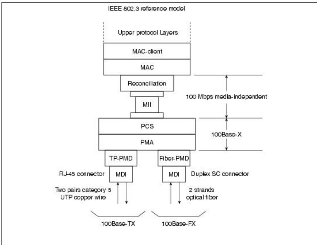
The 100Base-X encoding procedure is based on the earlier FDDI optical fiber physical media-dependent and FDDI/CDDI copper twisted-pair physical media-dependent signaling standards developed by ISO and ANSI. The 100Base-TX physical media-dependent sublayer (TP-PMD) was implemented with CDDI semiconductor transceivers and RJ-45 connectors; the fiber PMD was implemented with FDDI optical transceivers and the Low Cost Fibre Interface Connector (commonly called the duplex SC connector).
