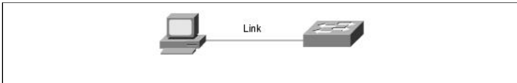
Figure: Example Point-to-Point Interconnection
