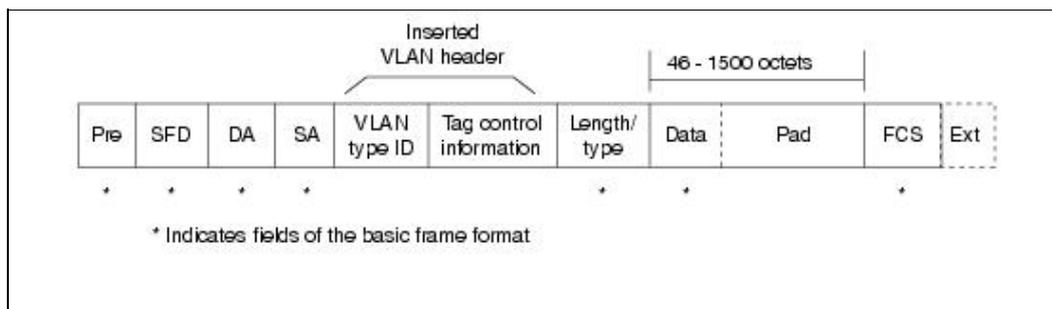
The VLAN header consists of two fields:
