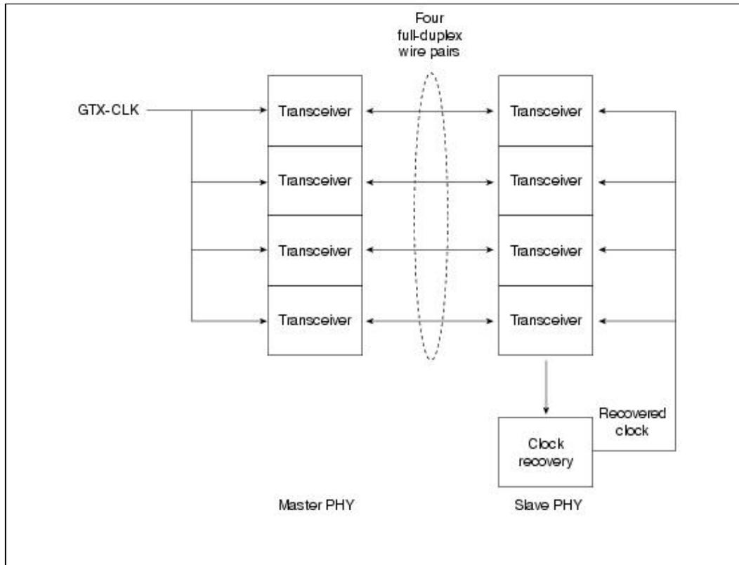
Each transmitted frame is encapsulated with start-of-stream and end-of-stream delimiters, and loop timing is maintained by continuous streams of IDLE symbols sent on each wire pair during interframe gaps. 1000Base-T supports both half-duplex and full-duplex operation.
