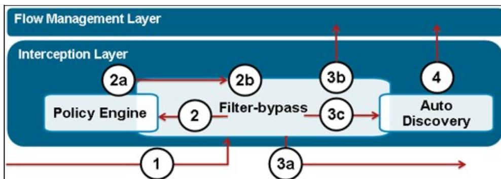
1. A SYN packet on a flow enters the system. This packet is routed to the filter-bypass module.
