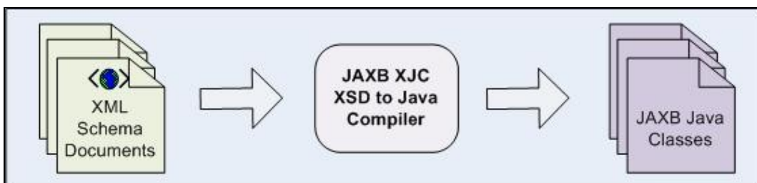
Figure 1: Running the XJC (JAXB Schema compiler) on CUE PI XML schema
