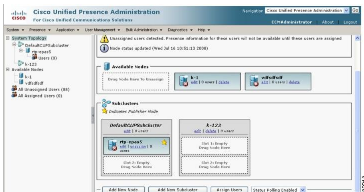
Figure: Cisco Unified Presence System Topology Navigation
