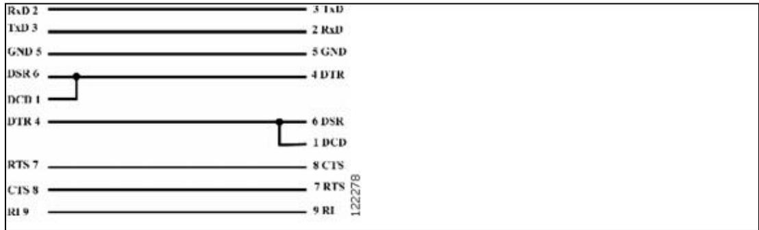
2. Connect one end of the null modem cable to the COM 1 port on the CPU card in the front of the Cisco Unified MeetingPlace Audio Server.
