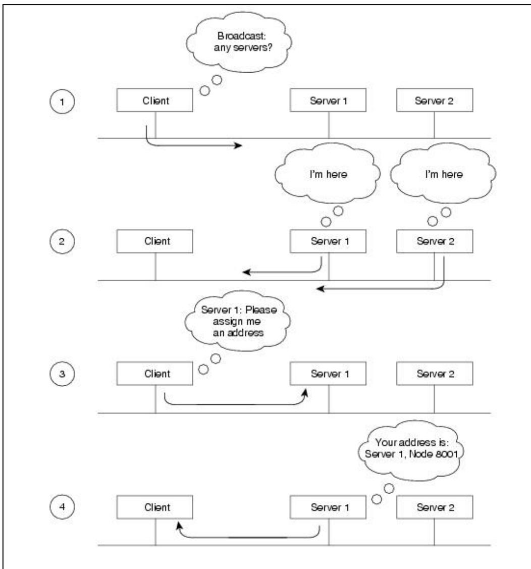
Dynamic address assignment is not unique in the industry (AppleTalk also uses this process), but it certainly is not as common as static address assignment. Because addresses are chosen exclusively by a particular server (whose address is unique as a result of the hardware key), very little chance exists for duplicating an address. This is fortunate because duplicate addresses could cause potentially devastating problems for
